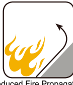
Reduced Fire Propagation NF C32-070-2.2(C1) IEC60332-3-24 EN50266-2-4
