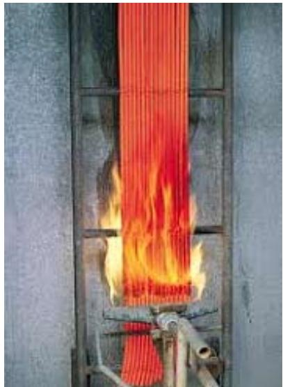
EN 60332-3-10:2009 / BS EN 60332-3-10:2009 / IEC 60332-3-10 ed1.1 / DIN EN 60332-3-10:2009 / VDE 0482-332-3-10:2010-08 – Common test methods for cables under fire conditions. Tests on electric and optical fiber cables under fire conditions - Part 3-10: Test for vertical flame spread of vertically mounted bunched wires or cables.
