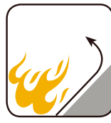
Reduced Fire Propagation NF C32-070-2.2(C1) IEC60332-3-24/EN50266-2-4
